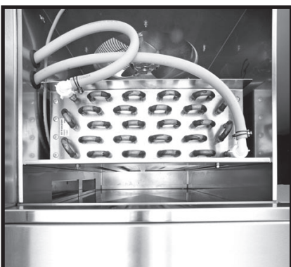
Hose down condensers.
