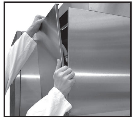
Clean once a month: Remove the front panel of the condenser hood.
