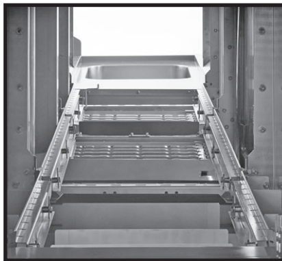
Hose down and clean the interior of the machine (particularly the bottom of wash and prewash tank) to avoid any waste remaining.
